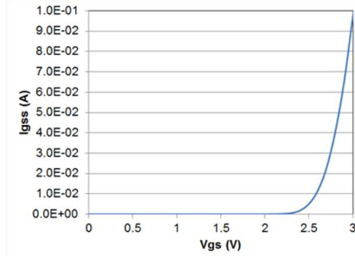
Figure 2. Gate Current vs. V<sub>GS</sub>
